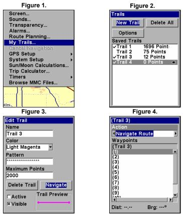
Navigate a trail menu sequence: Fig. 1, My Trails command. Fig. 2, Trails Menu. Fig. 3, Edit Trail Menu. Fig. 4, Edit Route Menu with Navigate Route command highlighted for Trail 1. A trail is always converted to a "route" when you navigate the trail.
